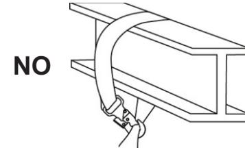
Diagram illustrating incompatible connections. The left side shows a compatible connection where a connector is correctly attached to a lanyard. The right side shows an incompatible connection where a connector is incorrectly attached to a metal beam, labeled 'NO'.
