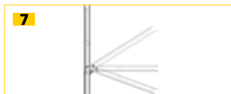
7 Montant rabattable Ø45 mm H : 1105 mm - articulation alu WV8201105F
