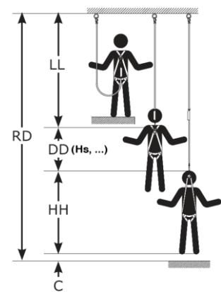
The calculation of the Required Fall Clearance Distance (RD) includes espacialy but without restriction:
