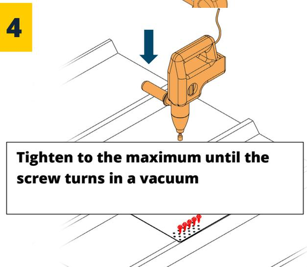
**Tighten to the maximum until the screw turns in a vacuum**
